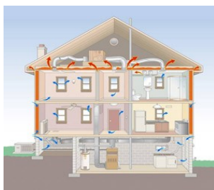
Heat escaping through air leaks and poor insulation can warm your roof, melt snow, and lead to ice on your roof.
