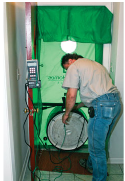
Figure 7. The technician verifies the correct operation of a new furnace and water heater (left) and documents the safety of the new kitchen range (below left). A final blower-door test (below) indicates the increase in house airtightness, from 3,600 CFM-50 to just over 1,900 CFM-50.
