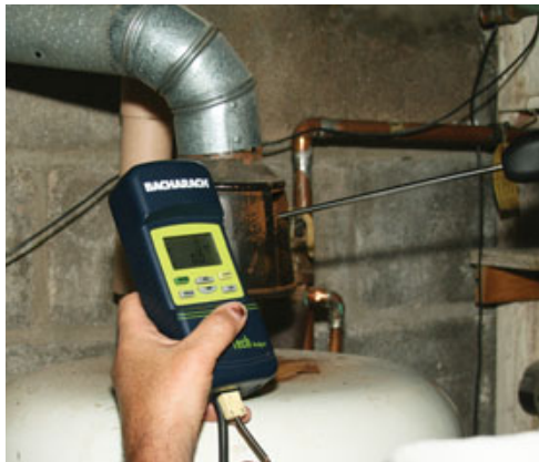
Figure 1. After drilling holes to insert sensor probes in the appliance flues (top left), the advisor uses a combustion analyzer to check for complete combustion in the furnace and water heater (top right). With doors and windows shut and all exhaust fans in the building operating, he uses a manometer to check the draft (bottom left); he is also required to check gas piping for leaks (bottom right).
