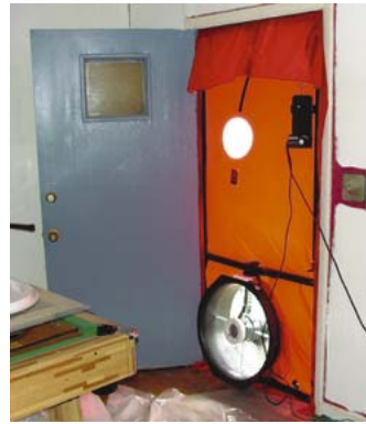
A blower door is easy to set up and instrumental in detecting leakage problems.
