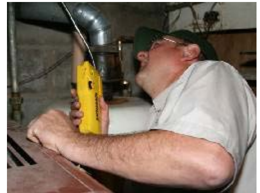
Bill Meadows checks a basement for gas leaks.
